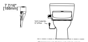
\*The 3-prong cord on the Washlet is on the right side and is 4' long. The GFCI outlet needs to have120V, 10amps.
