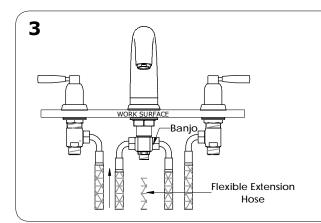
The supplied extension hose is to be fitted to the banjo as shown in the diagram.
