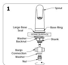
Place backnut onto shank and tighten to underside of worksurface.
