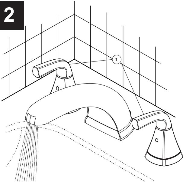
Turn faucet handles (1) all the way on. Turn on hot and cold water supplies and flush water lines for one minute.
