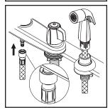
(4) Guide the side spray hose through the side spray holder. Insert the side spray hose quick connect adapter into faucet outlet end, push until a "click' is heard. Pull side spray hose downward to test engagement.
