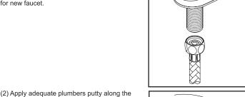
(5) When using stainless steel braided faucet supply hose; this faucet requires one end of the supply hose to have a 1/2" female IPS connection. The other end of this supply hose must match the thread on the water supply valve under your sink. Once you've identified the required size, carefully follow the manufacturer's installation instructions for each hose.
