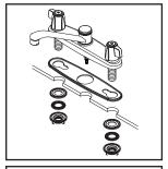
(2) Apply adequate plumbers putty along the boundary of base gasket. Align faucet with mounting holes and place faucet on the sink. Slide washers on shanks and secure the locknuts to the shanks from underneath the sink. Go to step (5) if faucet is without side spray.
