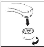
(6) Important: After installation is complete, remove the aerator. Turn on the water and allow both hot and cold water to run for at least one minute each. While water is running, check for leaks. Turn off the water and replace the aerator when finished.
