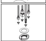
(2b) With flat side of the locknut facing down and the steel washer inside the locknut please follow the order as the drawing shows to insert flex hoses through the center hole of the locknut from underneath the sink.
