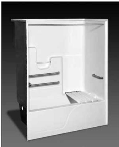
**Specification** – Oasis one-piece, 60 x 32-inch deep, FRP gelcoat bathtub model TS-6032 ABF (17.25-inch apron) having a factory-equipped package in compliance with 2010 ADA Standards for Accessible Design. Package includes 2-horizontal bars on back wall, single horizontal bar on head end wall, horizontal bar on control wall, REMOVABLE in-tub seat at head end and shower curtain rod.
