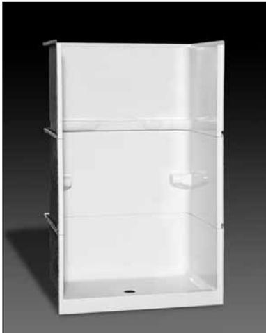
**Specification** – Oasis 3-piece FRP gelcoat shower compartment, SH3P-4832, offered in a standard 4-inch or 6-inch (ABF) dam configuration. ActivLife package includes factory applied, 3-wall, mid-level wrap reinforcement, exceeding (HUD/FHA) 'Fair Housing' requirements.
