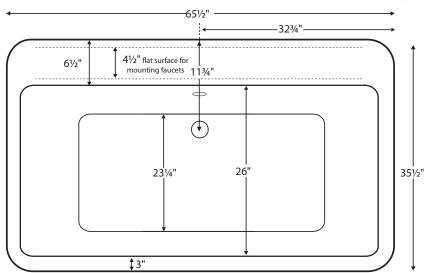
Features a 4.5" wide flat deck surface on the drain side for mounting faucetry.
