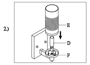
Step.2: Place the candle tube(D) and glass (E) on the socket
