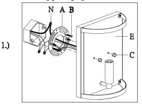
Step.1: Remove mounting bracket (A) from fixture and install to electrical box.
