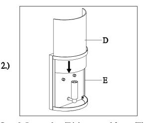
Step 2: Insert glass(D) into metal frame(E)
