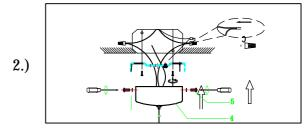
Step.2: Wire fixture to wires in outlet box. Green wire is for Ground. Secure canopy (B) to mounting bracket using screws on the sides of the canopy.
