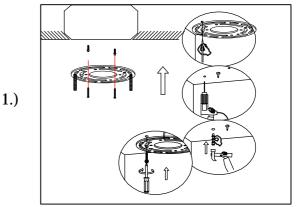
Step.1: Remove Mounting Bracket (A) from Canopy to install to electrical box
