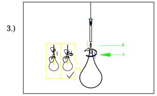
Step.3: Install G9 bulb (E) provided. Gently turn glass (F) onto socket (D) to secure.
